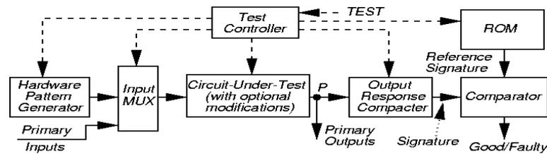
Fig.1 Block diagram of BIST
