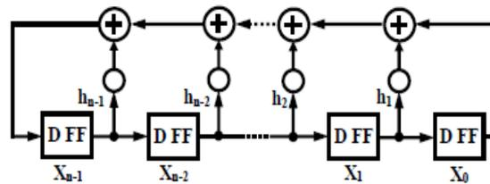
Fig.2 Standard LFSR circuit
