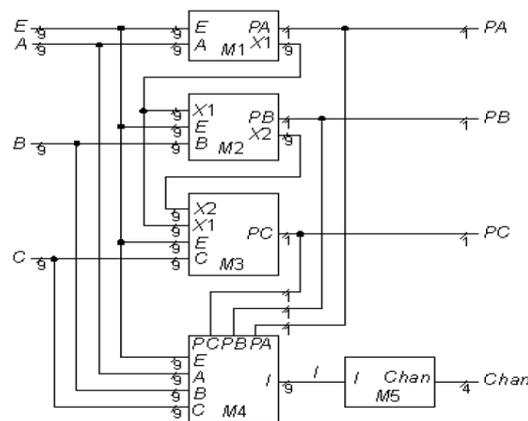
Fig. 3 C432 Combinational Circuit
