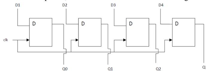
Fig 4: SIPO using MBFF
