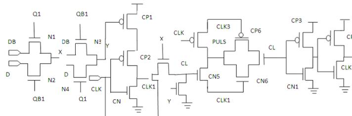
Fig 3.1(a) clock gated pulse generator
