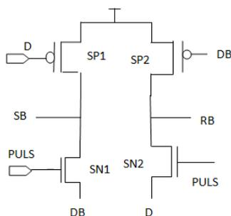
Fig 2.4.1(b) sensing stage
