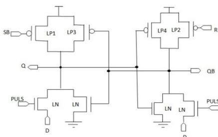
Fig 2.4.1(c) symmetric latch
