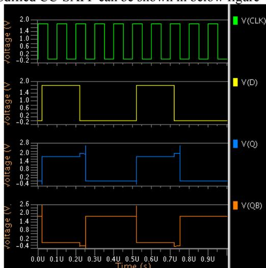
Fig4.1: simulated wave form of modified CC-SAFF
