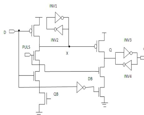
Fig 2.1(b) Static latch
