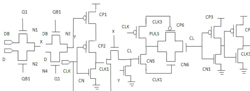
Fig 2.4.2(a): clock gated sense amplifier flip-flop pulse generating stage
