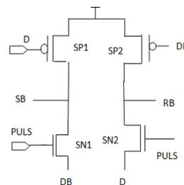
Fig 3.1(b) sensing stage
