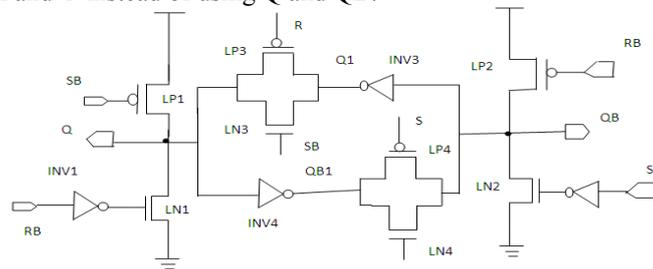
Fig 2.4.2(c) latching stage
