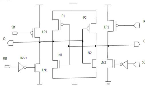
Fig3.1(c) latching stage
