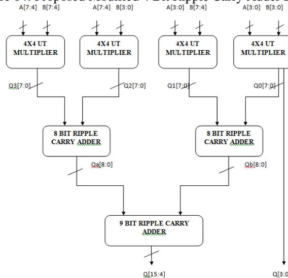
Figure 15: UT 8x8 Ripple Carry Adder Design
