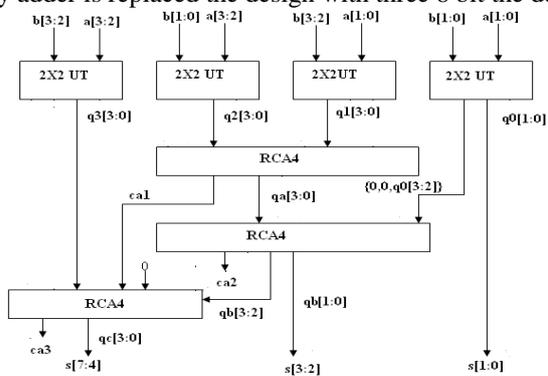
Figure 16: Proposed UT 4x4 Ripple Carry Adder
