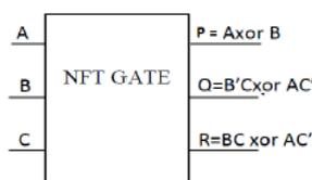
Figure 8: Block diagram of NFT Gate.
