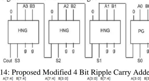
Figure 14: Proposed Modified 4 Bit Ripple Carry Adder Design.
