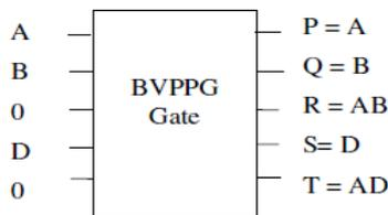
Figure 6: BVPPG Gate producing product terms and duplication of the inputs.
