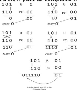
Figure 9: Urdhva Tiryakbhaya Procedure for Multiplication.
