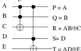
Figure 5: Toffoli Gate representation of BVPPG Gate
