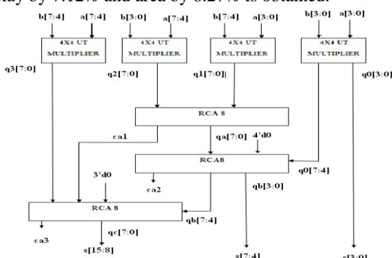
Figure 17: Proposed UT 8x8 Ripple Carry Adder
