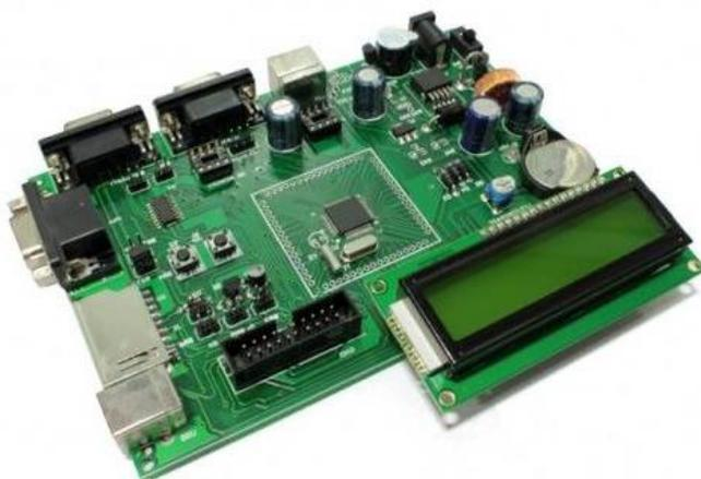
**Fig3:** ARM7 Processor Integrated with accessories
