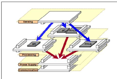
Fig.3. An Illustration of modular Structure of WSN Nodes [8]
