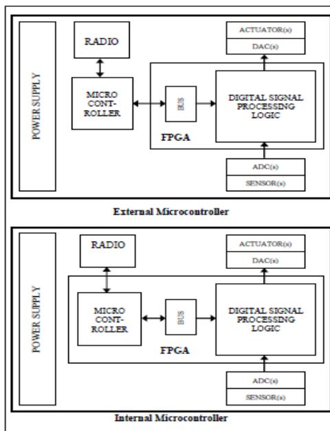
Fig.1. An FPGA-based WSN node. In both cases, FPGA is used for digital signal processing. In the first case, an external microcontroller is used to manage radio communication and the operating system. In the second case, the microcontroller is implemented into the FPGA [17]
