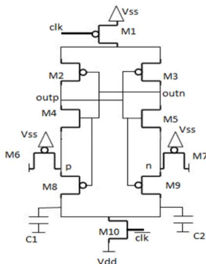
Fig. 2 Pre-amplifier based clocked comparator
