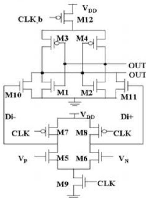
Fig. 1 Double tail comparator
