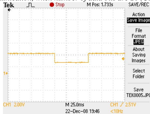
Figure 8: Waveform – communication, when number of data bits are 44 (Communication Delay = 72.5 ms)
