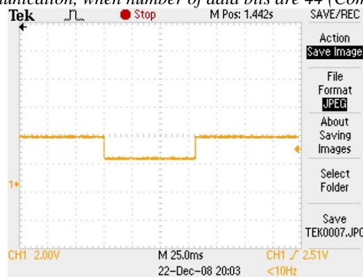
Figure 9: Waveform – communication, when number of data bits are 30 (Communication Delay = 80 ms)
