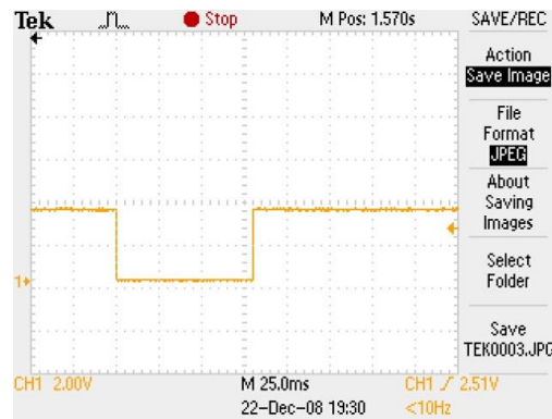
Figure 7: Waveform – communication, when number of data bits are 26 (Communication Delay = 80 ms)
