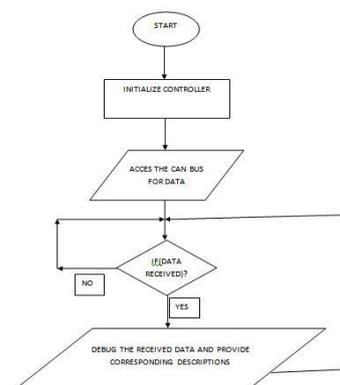
Fig.3 Flow chart for OBD Scanner
