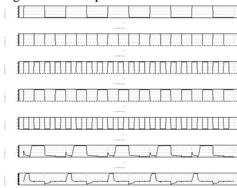
**Figure 6(b).** Simulated waveforms of ECRL
