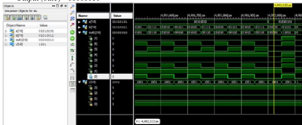
Fig 14:- Timing diagram of SUB operation
