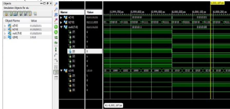
Fig 16:- Timing diagram of DEC operation
