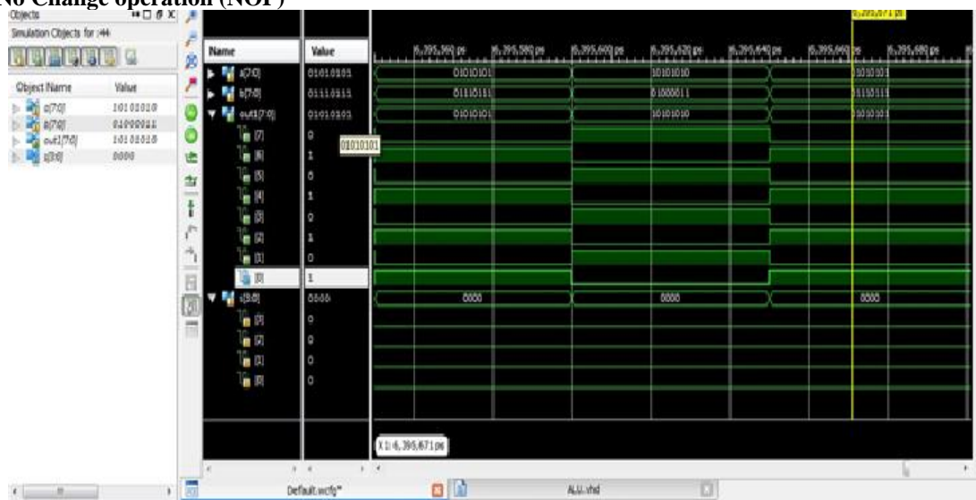
Fig:- 6 timing diagram of No change Operation (NOP)
