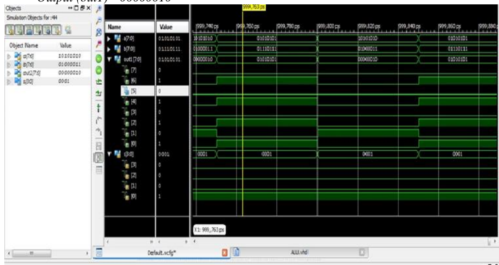
Fig 7:- Timing diagram of AND operation
