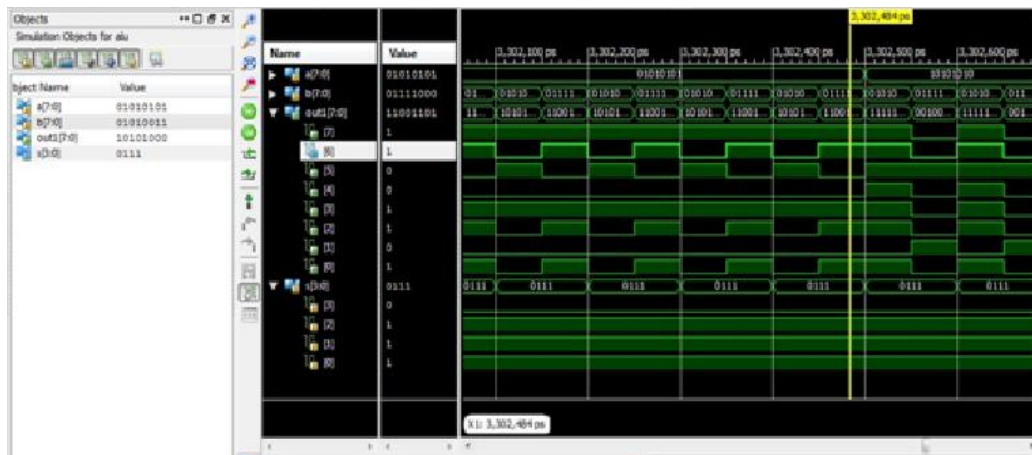
Fig 13:- Timing diagram of ADD operation
