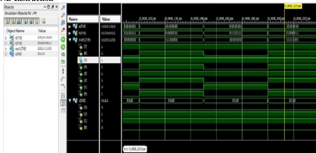
Fig 12:- Timing diagram of NAND operation
