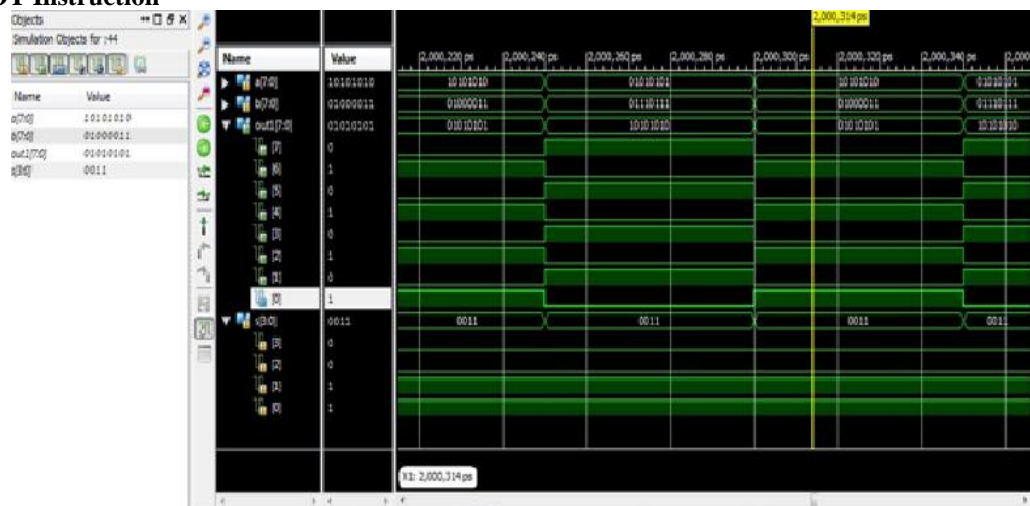
Fig 9:- Timing diagram of NOT operation
