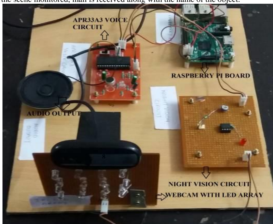
Figure (6): Hardware Implementation of the system
